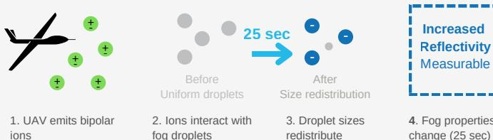
**The breakthrough finding:** Unipolar ion emission increased fog reflectivity with a peak response approximately 25 seconds after emission, indicating rapid redistribution of droplet sizes. The study used both clear-air and foggy-air conditions as controls, enabling robust analysis of the ionization effects. This represented the first time scientists had intentionally modified fog microphysics and radiative properties under natural atmospheric conditions using controlled ion emissions.
